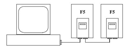
Host with InterBus-Option (PC, VME, SPS) KEB COMBIVERT F5 with InterBus-Operator
