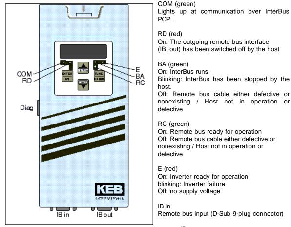
IB out Remote bus output (D-Sub 9- socket)
