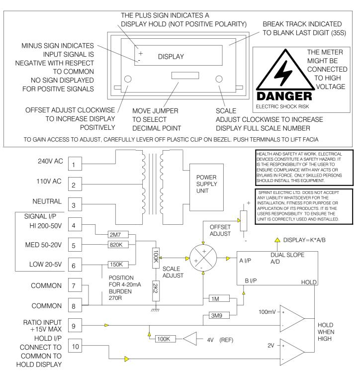
Choose signal input terminal 4, 5 or 6 to suit full scale range. The scaling preset will then span between 10% and 100% of the display range. All signal inputs are referred to COMMON on terminals 7 and 8.
